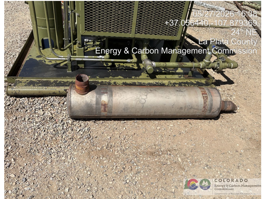
24. Muffler resting on ground. Unattached.
