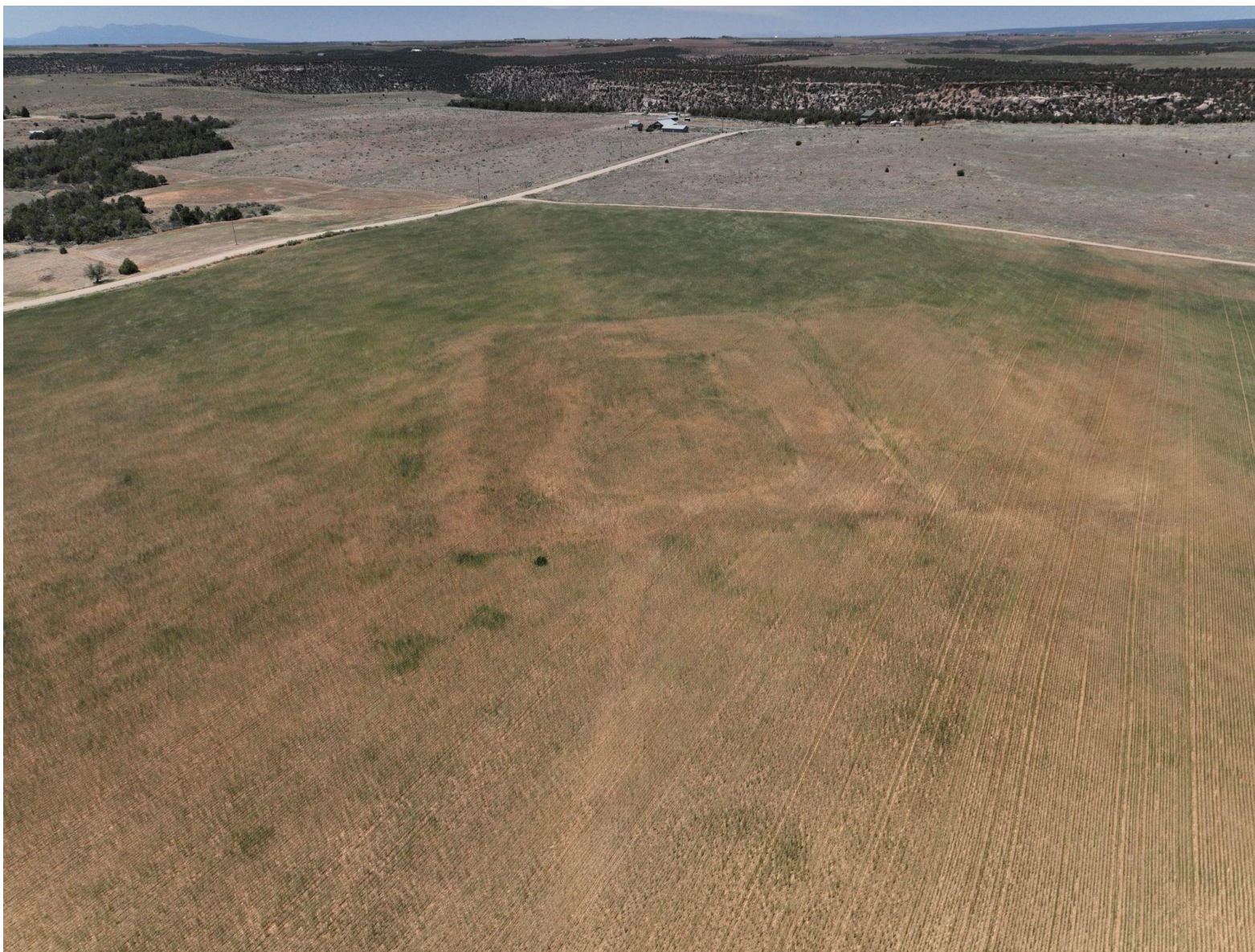
Photo 2. View of well pad and associated access road taken with a drone during the time of the inspection from the southern edge facing north. Note: stunting observed at well pad compared to reference areas, see photo 4.
