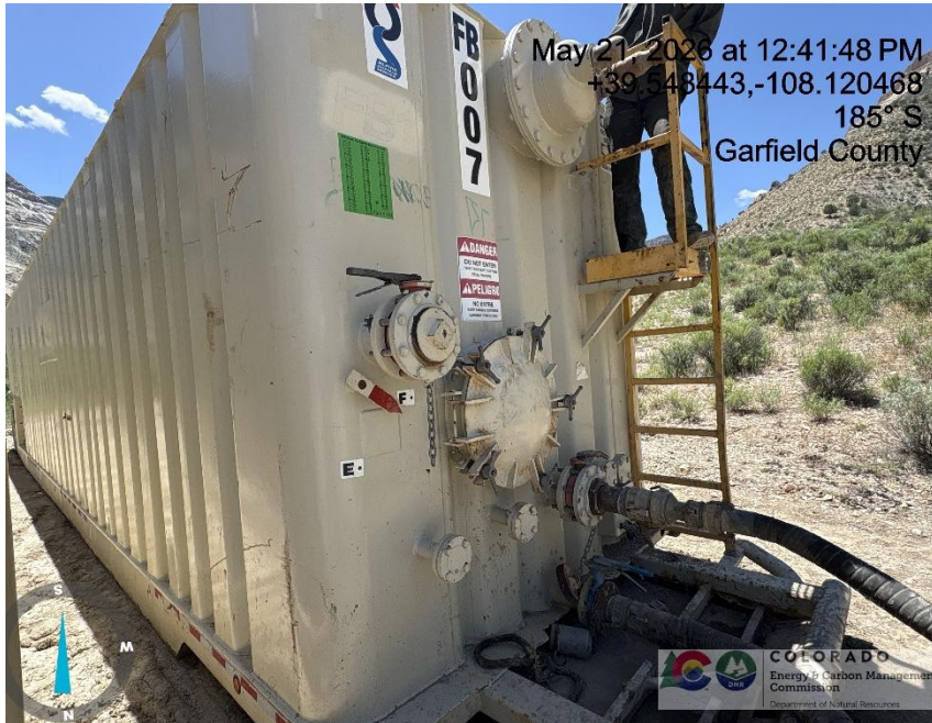
Photo # 1295 Frac tank lacks required labeling
