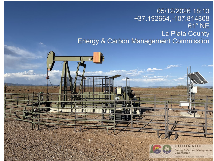
2. Wellhead, pump jack and solar telemetry behind steel cattle panel fence. There is also a black steel mesh cage around the drive portion of the pump jack.
