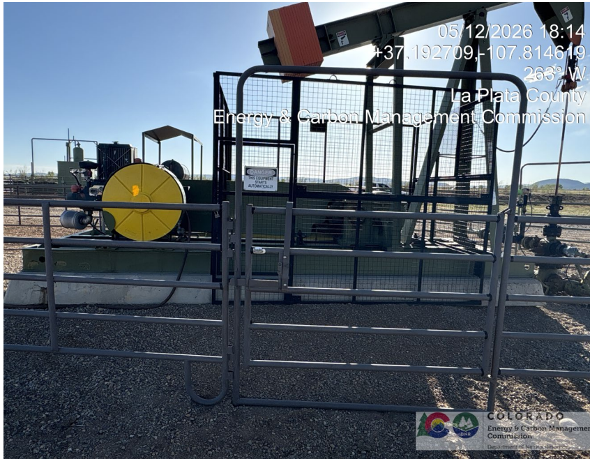
5. Well gas prime mover, pump jack, and wellhead.
