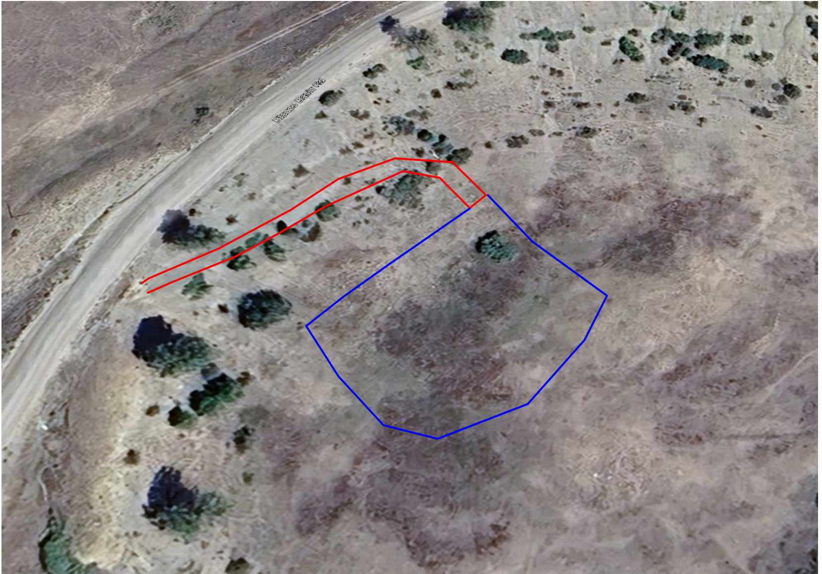
Photo 1. 2025 NAIP Imagery of the well pad (highlighted in blue) and associated access road (highlighted in red).
