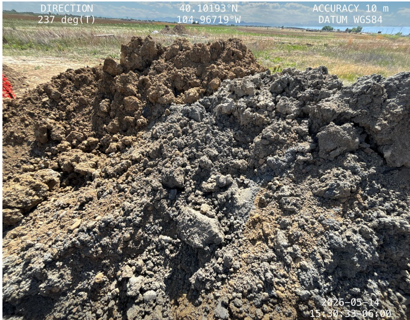
Discolored soil within stockpile
