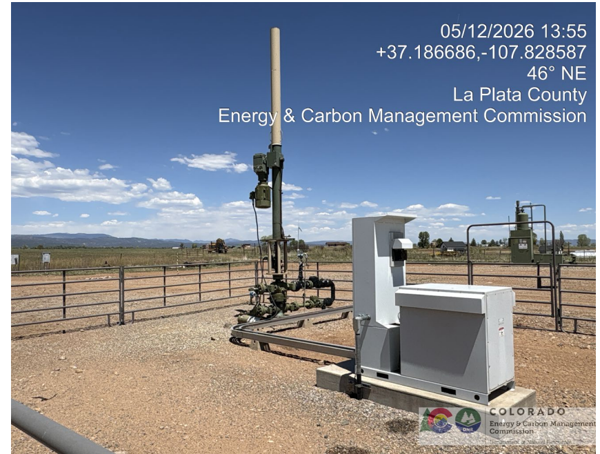
2. Wellhead, electric drive linear rod pump, electrical controls. Cattle panel fence.
