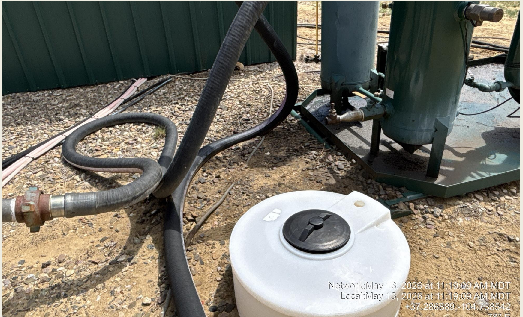
PHOTO 9: AREA OF IMPACTED SOIL NEAR COMPRESSOR SKID. AT TIME OF INSPECTION THIS EQUIPMENT IS NOT IN OPERATION HOWEVER IT APPEARS TO HAVE SIGNIFICANT OIL LEAKS THAT SHOULD BE REPAIR PRIOR TO PUTTING EQUIPMENT BACK IN USE. Conduct maintenance on equipment, cleanup stained material and review self inspection processes. COMPLY WITH RULE 1002,.(2).D CA DATE 6/13/2026.
