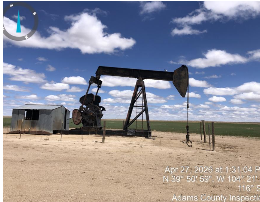
Photo #3 Pump jack.
