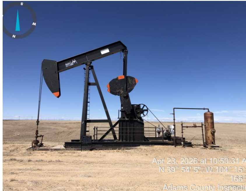
Photo #3 Pump jack.
