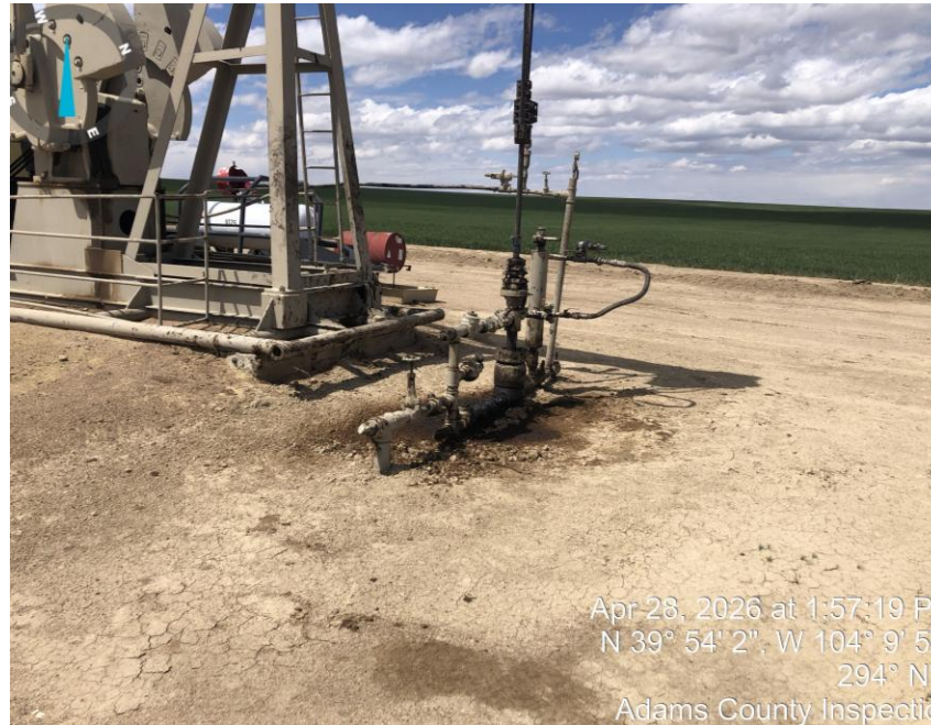
Photo #5 stained soil around well head.
