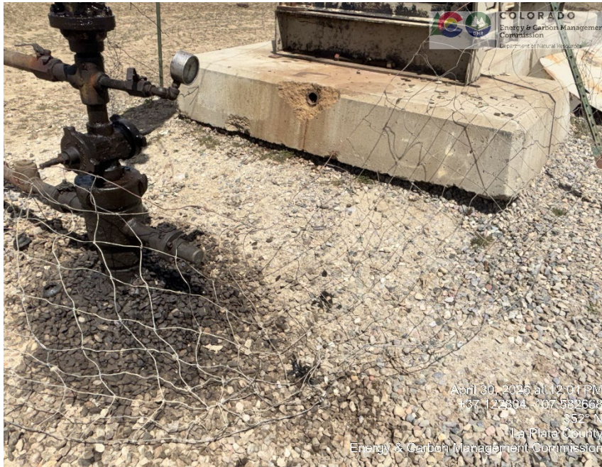
WELLHEAD LUBRICATION LEAK IMPACTED SOIL
