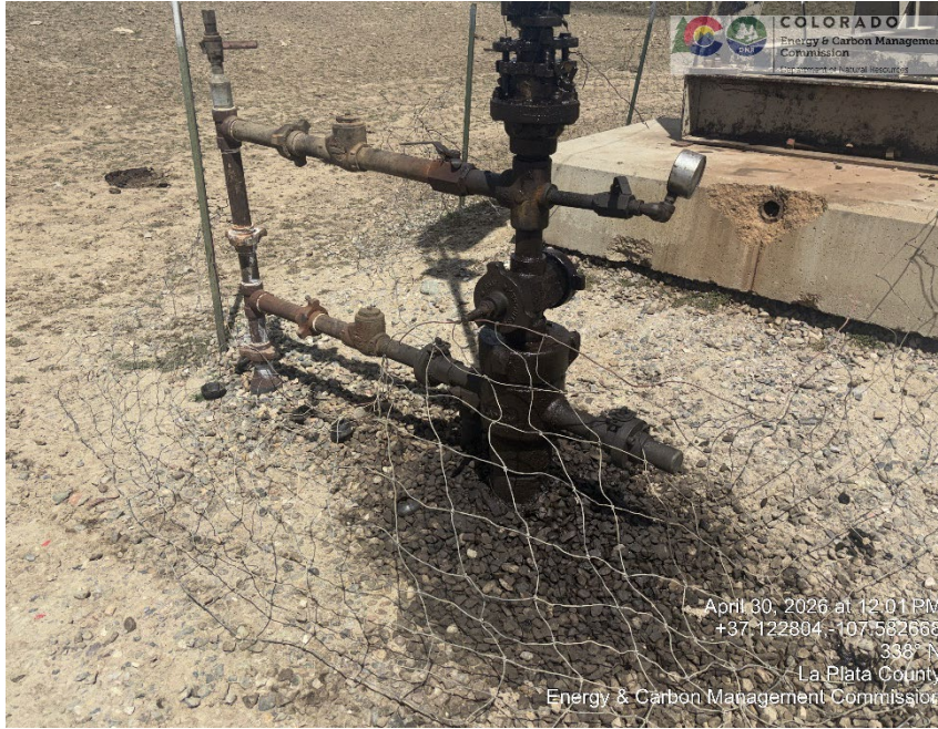
WELLHEAD LUBRICATION LEAK IMPACTED SOIL
