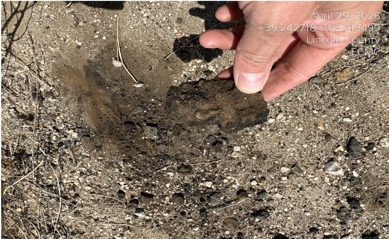
Photo 8. There is hydrocarbon impacts at the former tank battery that have become exposed at the surface..
