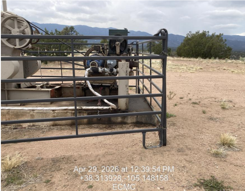
Photo 3: Oily buildup on pumping unit base
