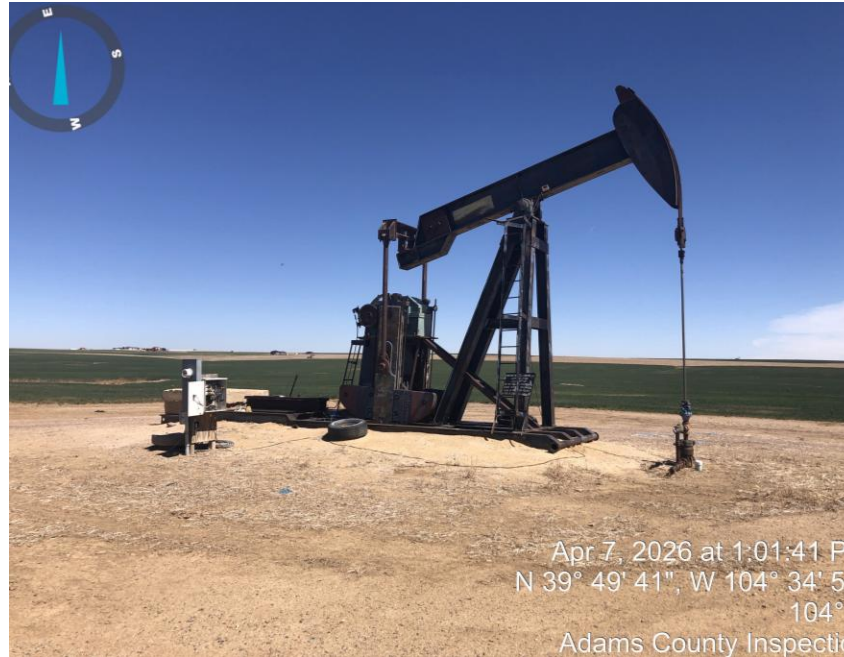
Photo #3 Pump jack.
