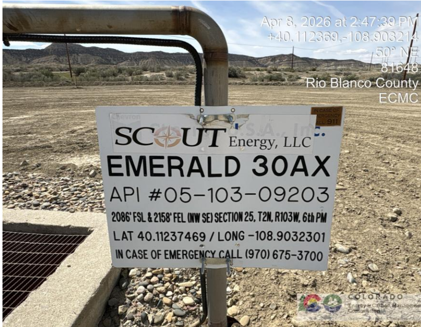
Photo # 4311 Wellhead sign lacks public road used to access the well
