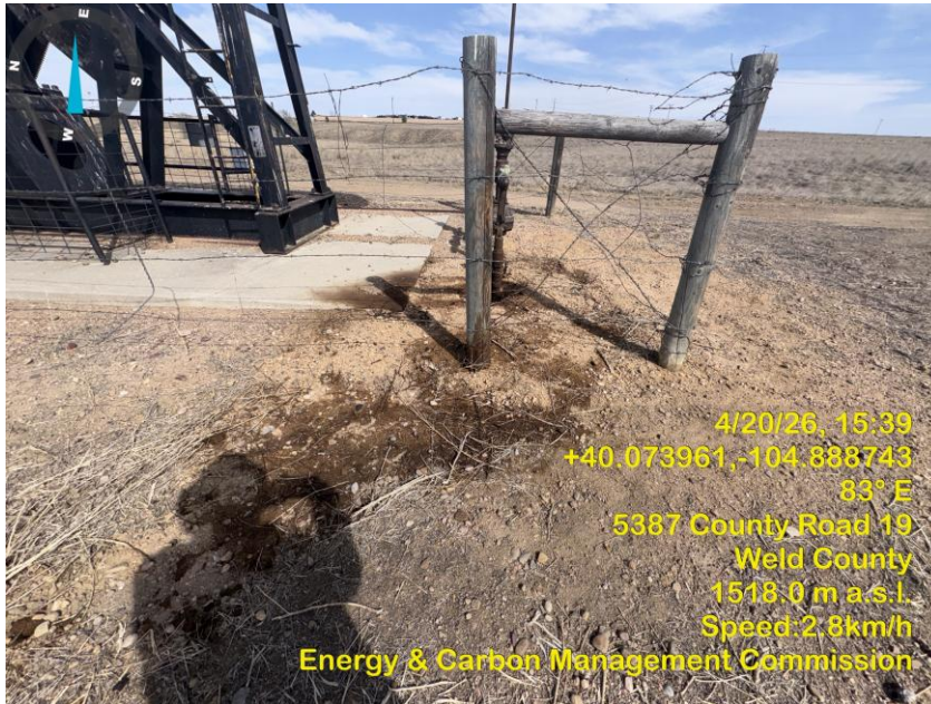
Photo 5 Stained soil by the wellhead.
