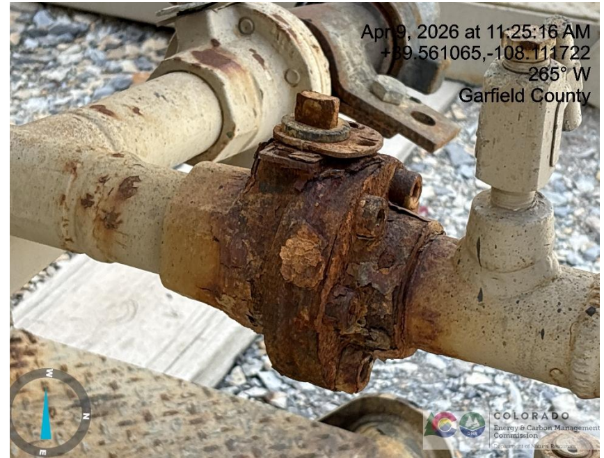
Photo # 6531 Mechanical Condition - Large amount of external corrosion visible on ball valve (N. PARACHUTE MF07C-4 C04 696 flowline)
