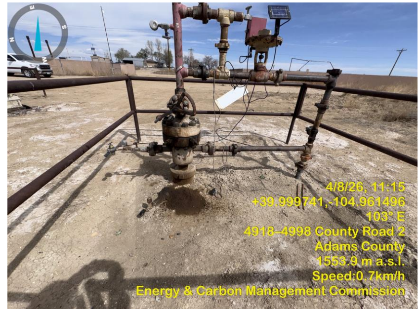
Photo 24 Stained soil by the bradenhead valve under the master valve..
