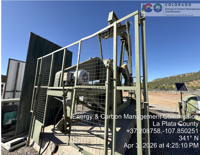
9. Pumpjack and electric prime mover.
