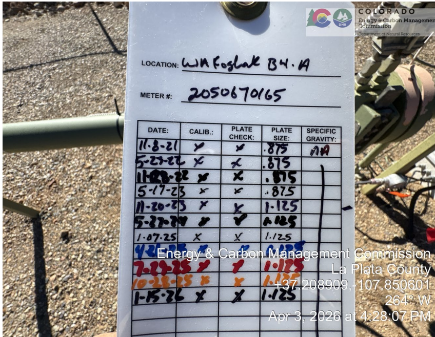
13. Meter calibration card dated 1/15/2026.
