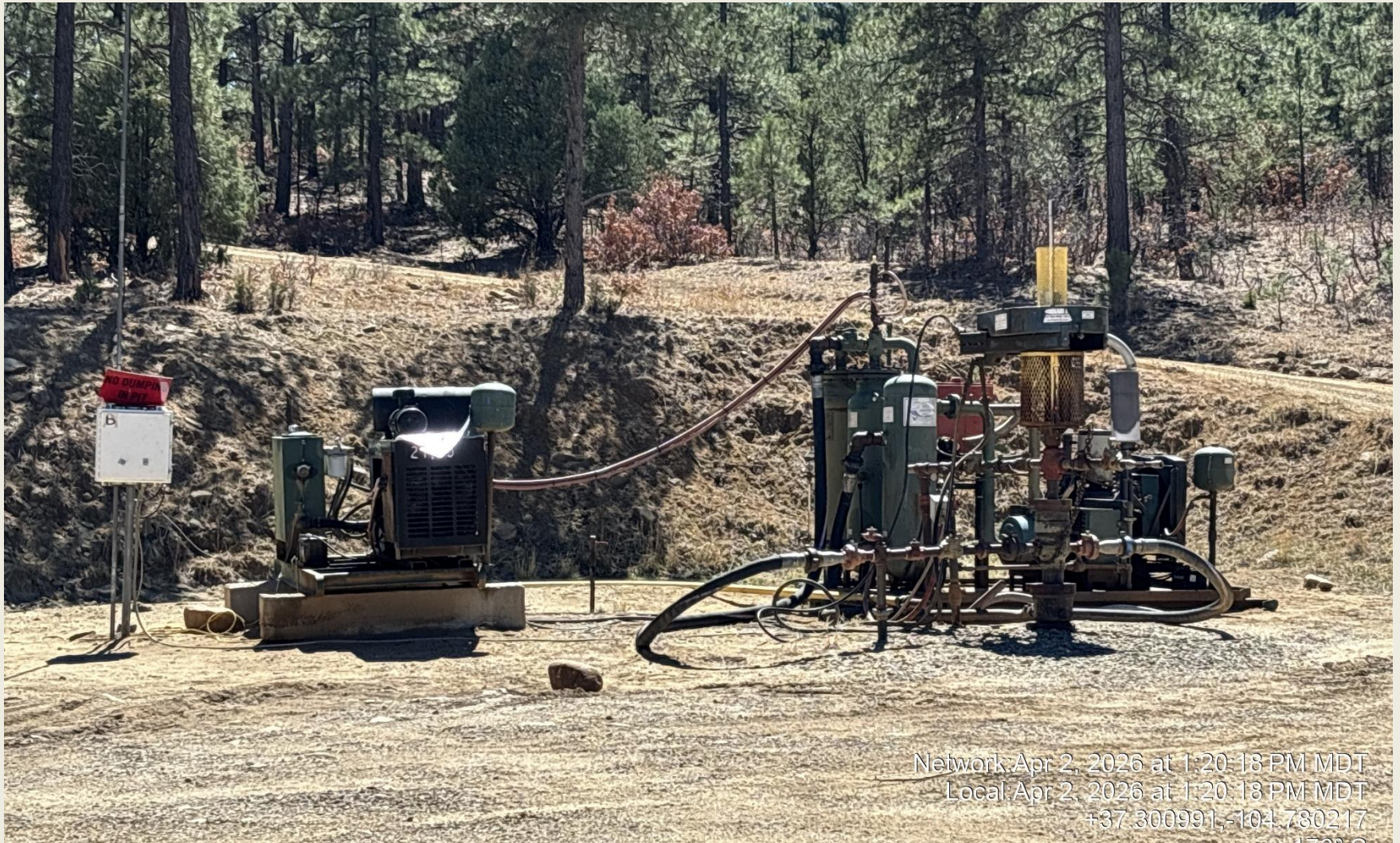
PHOTO 4: TR WELLHEAD AND EQUIPMENT. Vacuum pump observed on well without ECMC approval. Provide ECMC with documentation showing approval of use of vacuum pump. CA DATE 4/17/2026.
