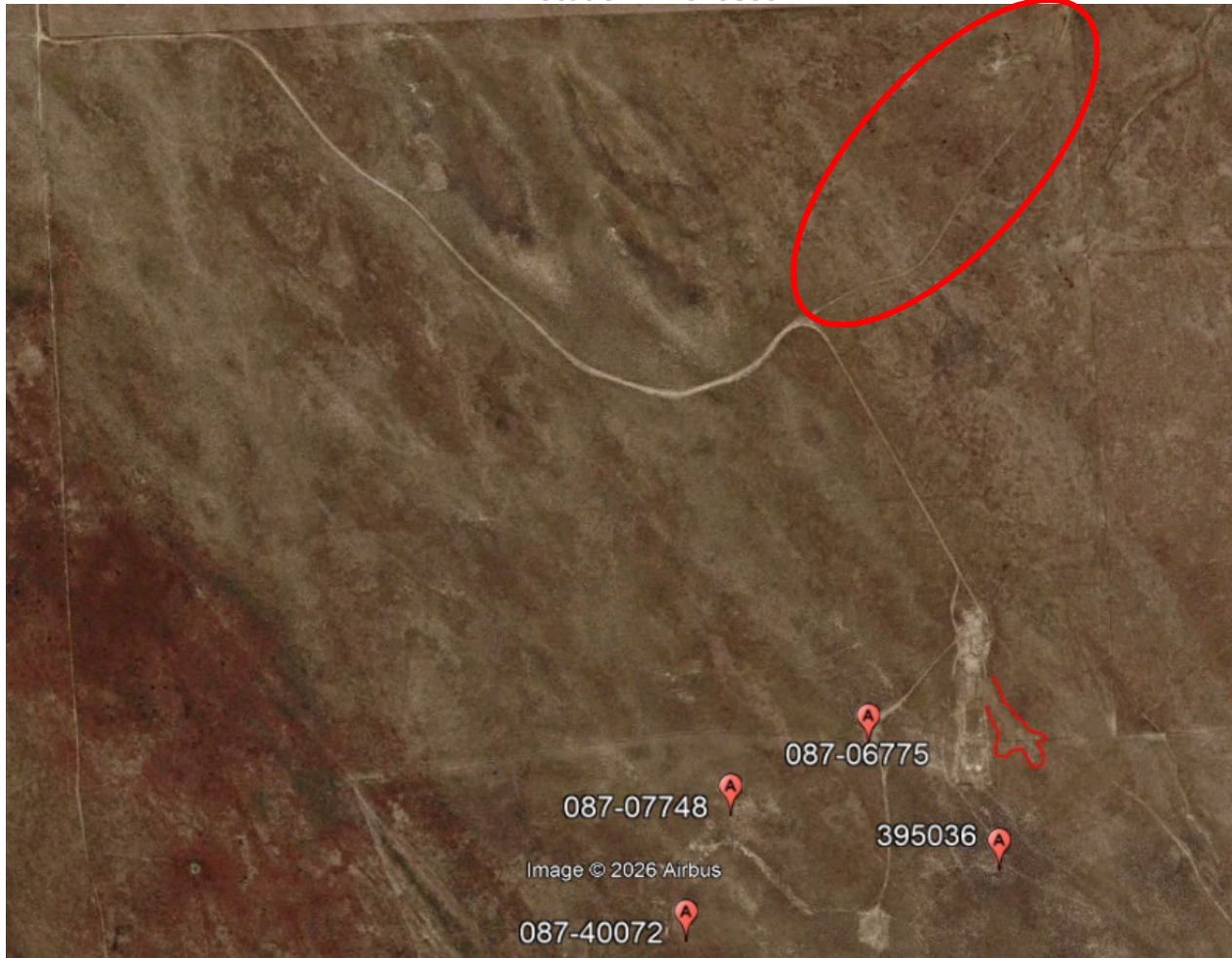
Photo 27. Google Earth satellite imagery showing the main lease road leading to the tank battery and Merino State 3 is still visible. The Northeastern section of the access road, circled in red, is progressing to final reclamation; however, the other section of the main lease road to the tank battery pits and well head is not and needs to be reclaimed. The site visit on February 11 confirmed that the main lease road was still visible and that reclamation had stalled.
