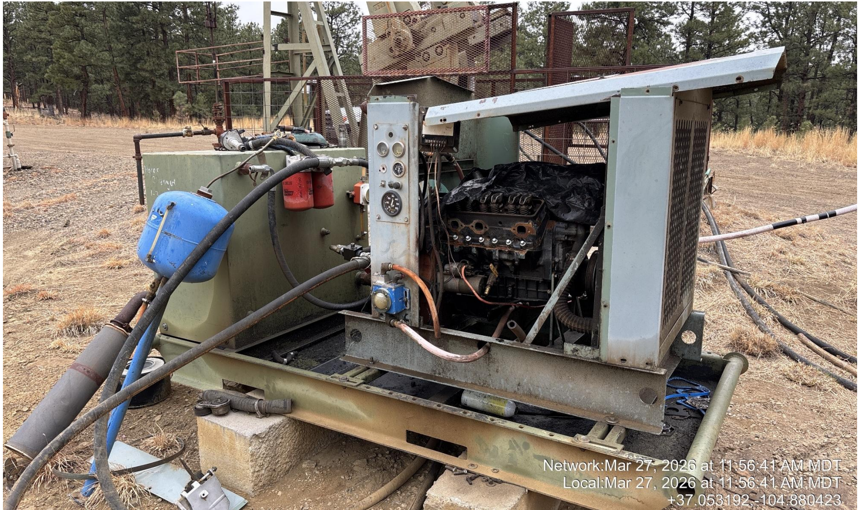
PHOTO 6: UNUSED EQUIPMENT (PRIME MOVER ENGINE SKIT IS NOT USABLE ON R WELL). THIS TYPE OF WORK CANNOT BE PERFORMED ON LOCATION. REMOVE UNUSED EQUIPMENT PER RULE 606. CA DATE 4/2/2026.
