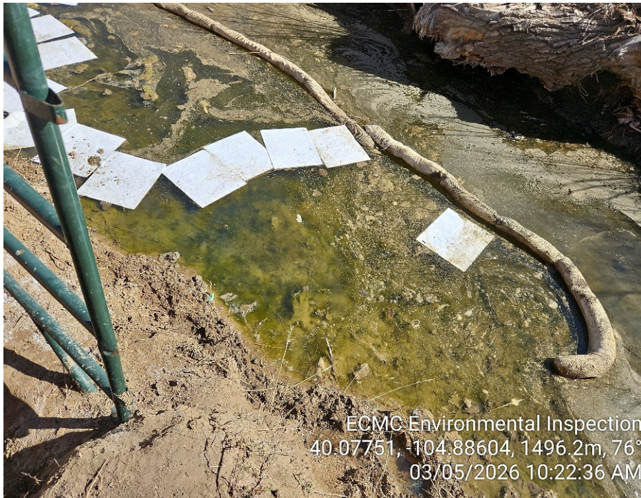
Photo 3 – Hydrocarbon sheen observed on Big Dry Creek. Booms and mats placed in Big Dry Creek have not been maintained and require replacement.
