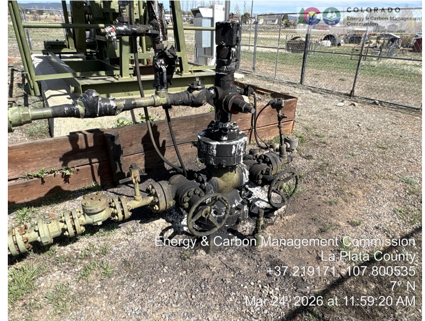
12. Wellhead with mineral crust and stained gravel beneath. Gas bubbles can be seen each time the polished rod gets near the bottom of each stroke. There is some produced water seeping, but no standing water on ground. Soil is stained from polished rod oil and mineral crust. Video of bubbles attached to report.
