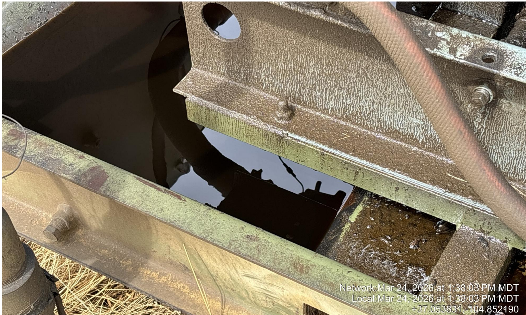
PHOTO 5: OILY WASTE INSIDE PRIME MOVER ENGINE SKID. DRAIN OILY WASTE REPAIR ALL LEAKS AND REMOVE IMPACTED SOIL PER RULE 1002..(2).D & 1002.f.(2)B, Comply with general provisions of the oil and gas act for wildlife protection AND SB-181. CA DATE 3/25/2026 FOR OILY WASTE, 3/30/2026 TO REMOVE IMPACTED SOIL.
