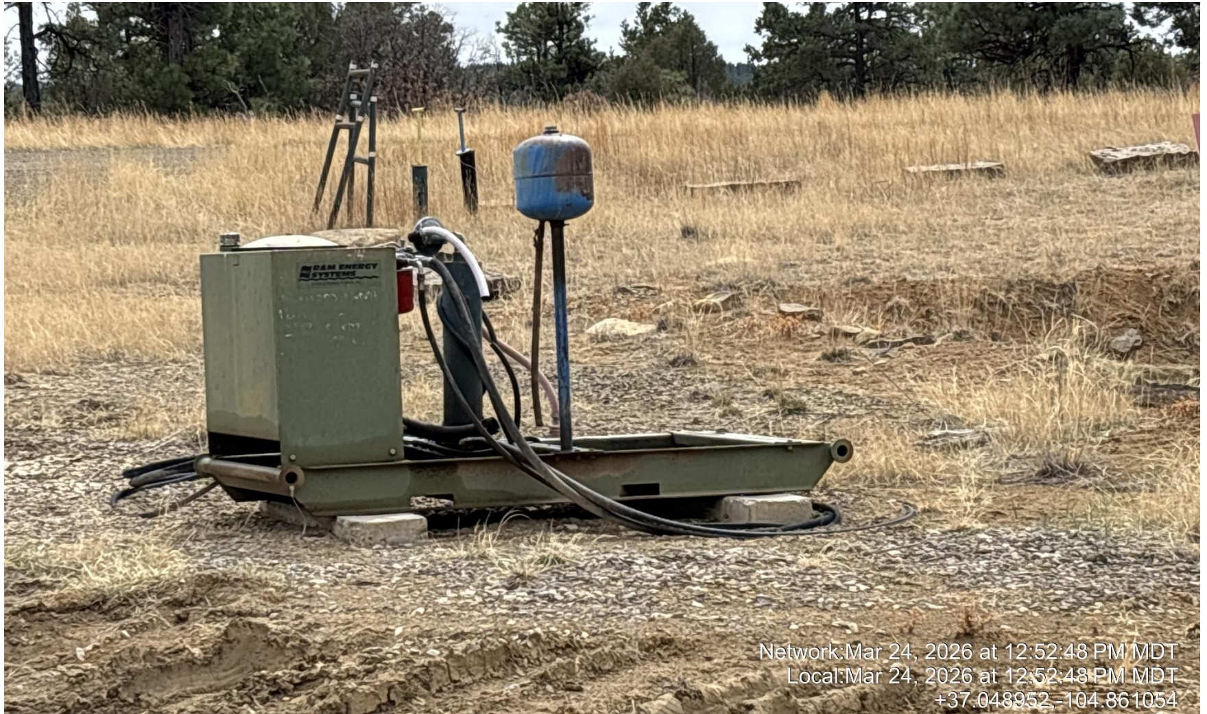
PHOTO 5: UNUSED EQUIPMENT (PRIME MOVER SKID WITHOUT ENGINE IS NO LONGER IN USE OR USEFUL). REMOVE UNUSED EQUIPMENT PER RULE 606. CA DATE 4/24/2026.
