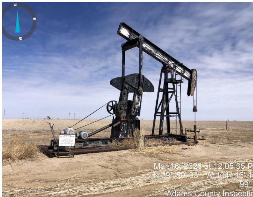
Photo #1 Pump jack.
