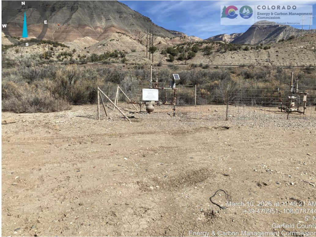
Subsidence of ground surface in front of GM 21-2
