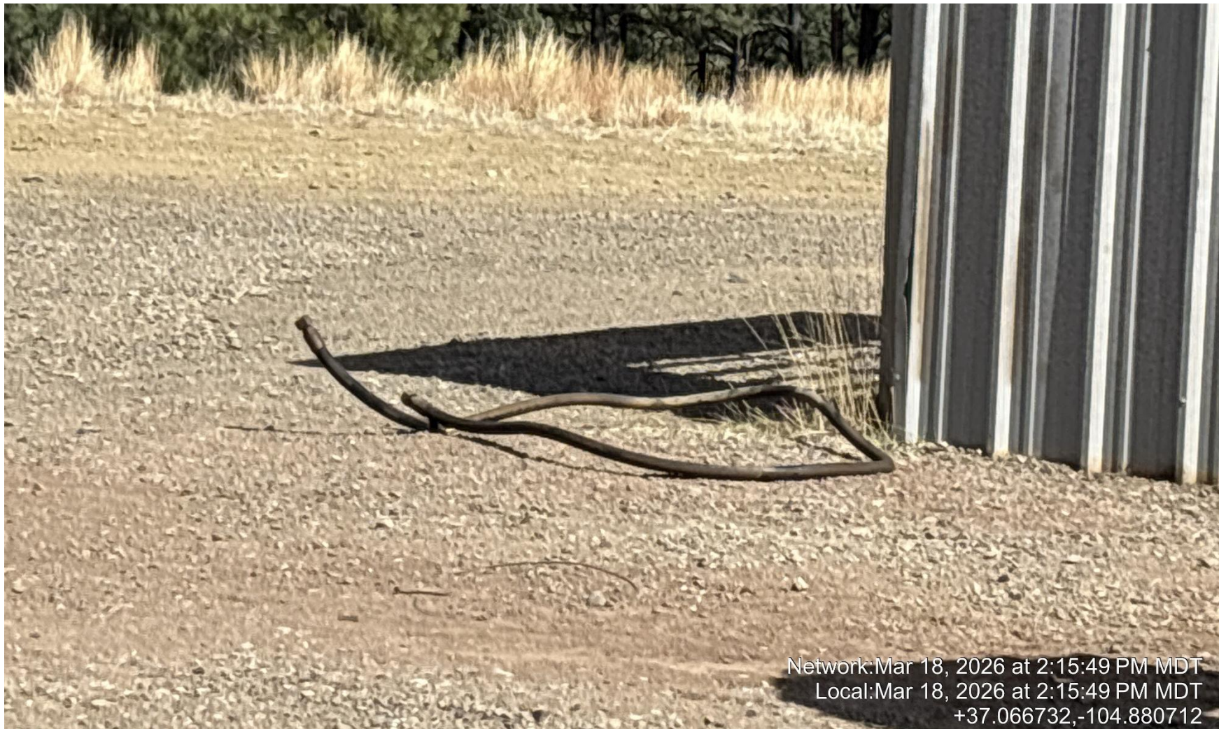
PHOTO 9: UNUSED EQUIPMENT (HYDRALIC HOSE NEAR PRIME MOVER SOUND WALLS). REMOVE UNUSED EQUIPMENT PER RULE 606. CA DATE 3/24/2026.
