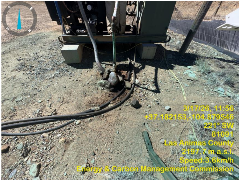
Photo 11 Stained soil by skid engine gas valve.
