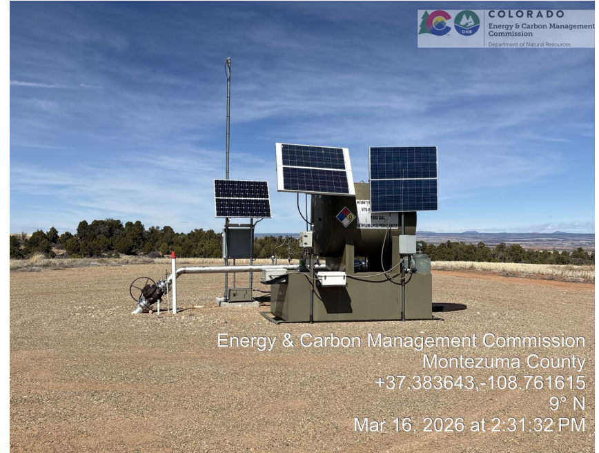
4. Wellhead, stainless flowline, 1000 gallon produced water/diethylene glycol tank atop secondary containment tank with expanded metal screen, and solar telemetry.
