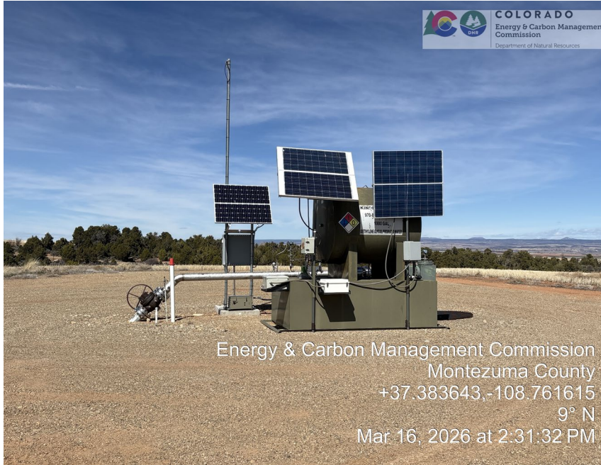
5. Wellhead, stainless flowline, 1000 gallon produced water/diethylene glycol tank atop secondary containment tank with expanded metal screen, and solar telemetry.
