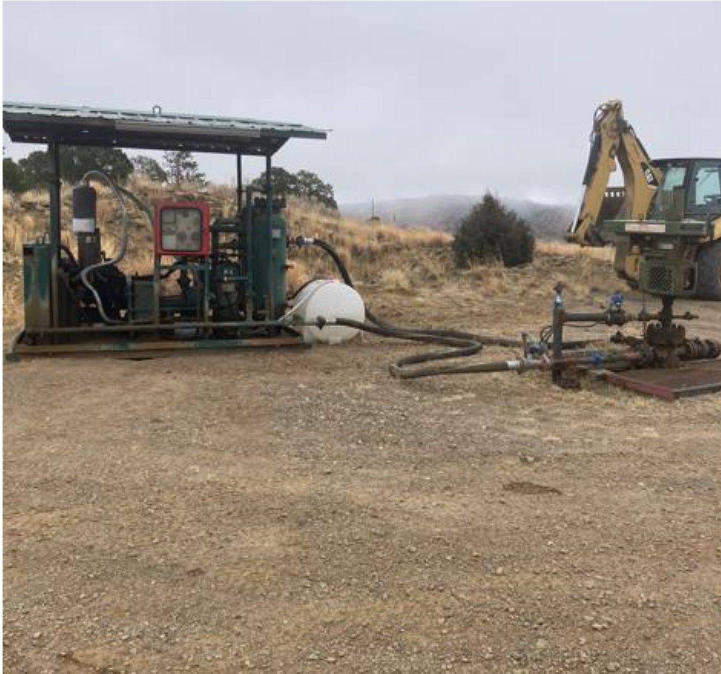
PHOTO 1: ALL SOIL STAINS HAVE BEEN REMOVED FROM LOCATION AND ALL OPERATING EQUIPMENT HAS RECEIVED MECHANICAL MATINTENANCE. THE UNUSED ENGINE AND SKID HAVE BEEN REMOVED FROM LOCATION. A CAP HAS BEEN PLACED ON THE OPEN VALVE TO PREVENT WILDLIFE ENTRANCE.
