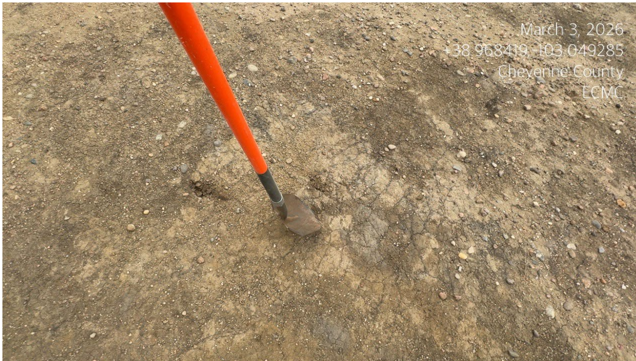
Photo 7. The soils in the area shown in the previous photo has very compacted soils that a shovel could not penetrate. Soils also appear to be discolored in this area.
