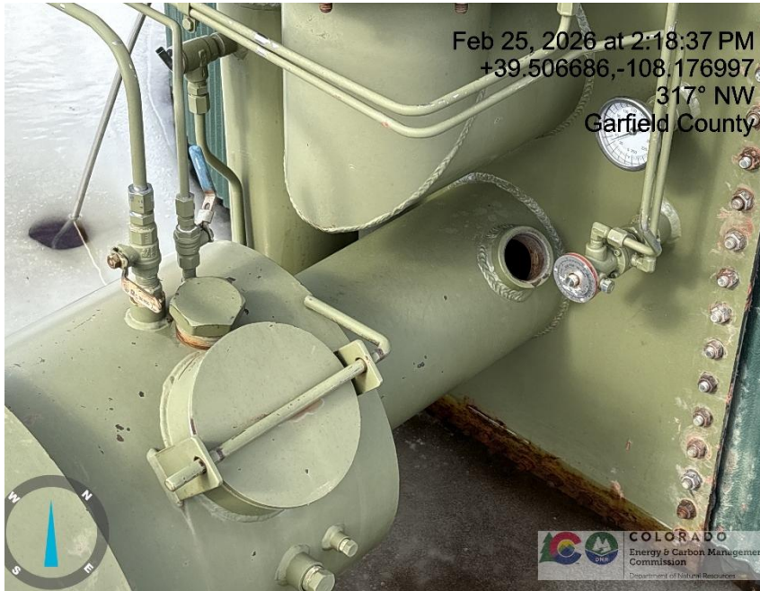
Photo # 4175 Open ended pipe on fire tube/wildlife hazard /available for entry by wildlife
