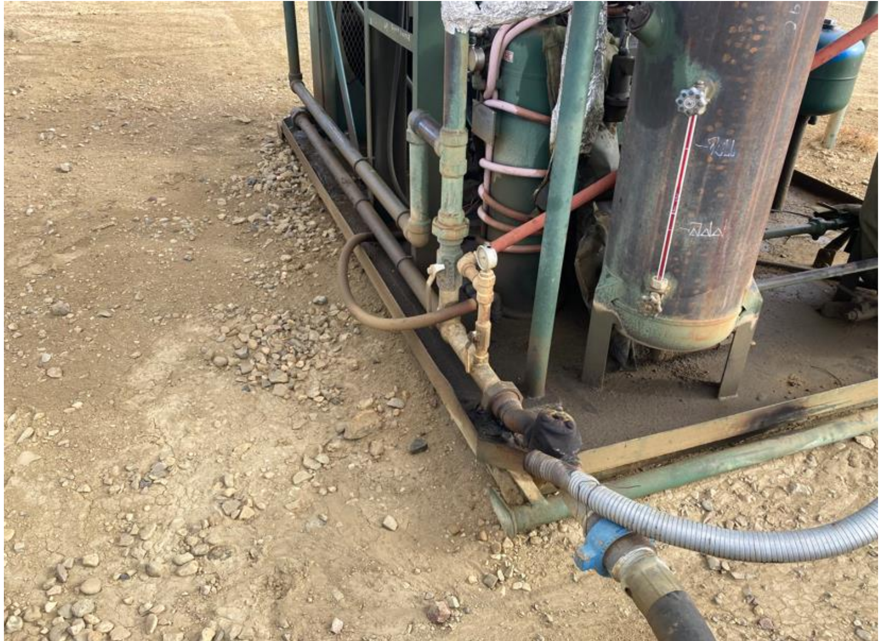
PHOTO 2: THE COMPRESSOR SKID HAS BEEN CLEANED AND ALL OPERATING EQUIPMENT HAS RECEIVED MECHANICAL MAINTENANCE. ALL IMPACTED SOIL ON LOCATION HAS BEEN REMOVED AND REPLACED WITH FRESH PAD MATERIAL.
