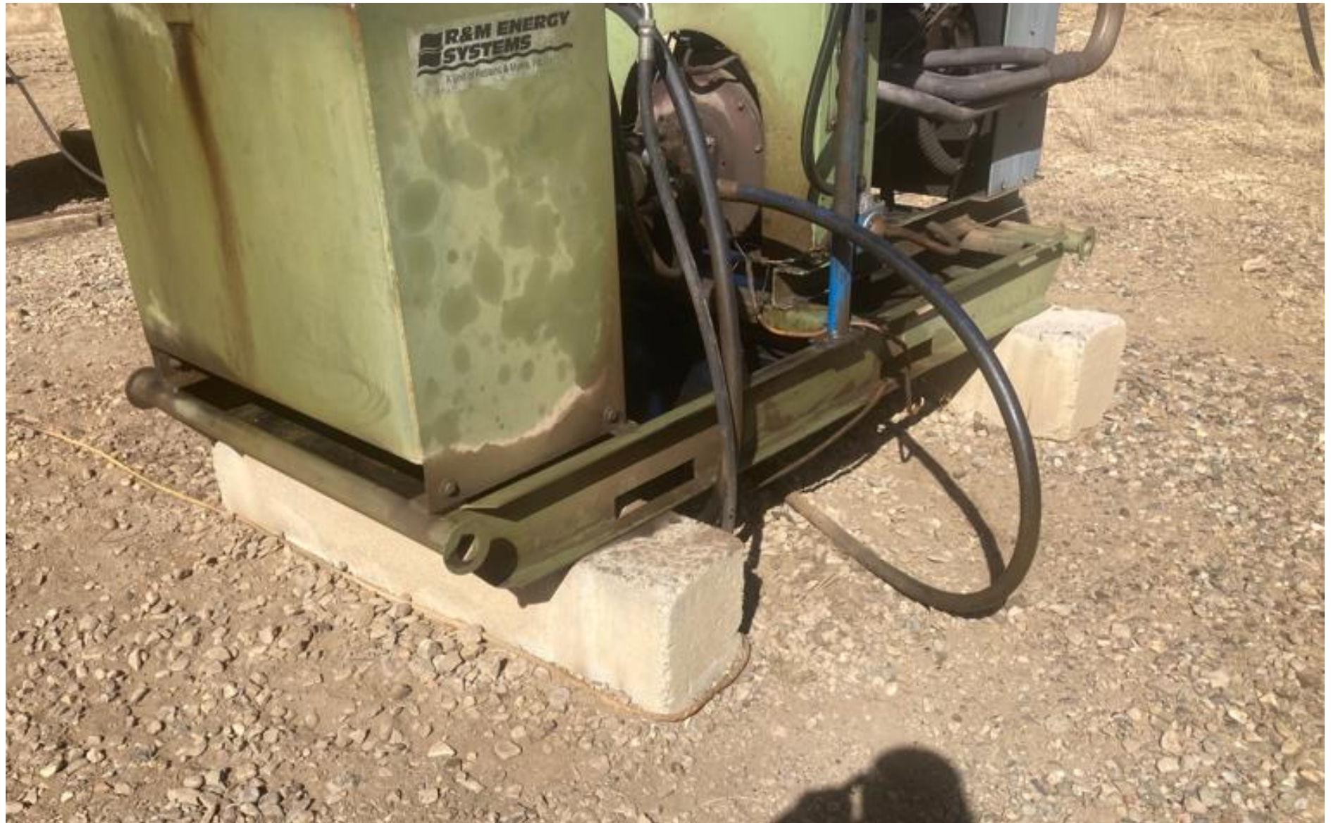
PHOTO 2: THE ENGINE SKID HAS BEEN CLEANED AND ALL STAINED SOIL HAS BEEN REMOVED FROM LOCATION. FRESH PAD MATERIAL HAS BEEN ADDED. ALL OPERATING EQUIPMENT HAS RECEIVED MECHANICAL MAINTENANCE.
