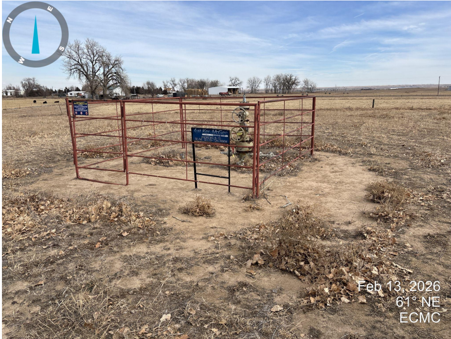
Photo 1. Looking east at the wellhead. Location size is reduced. Desirable perennial vegetation appears to be established in the interim area.
