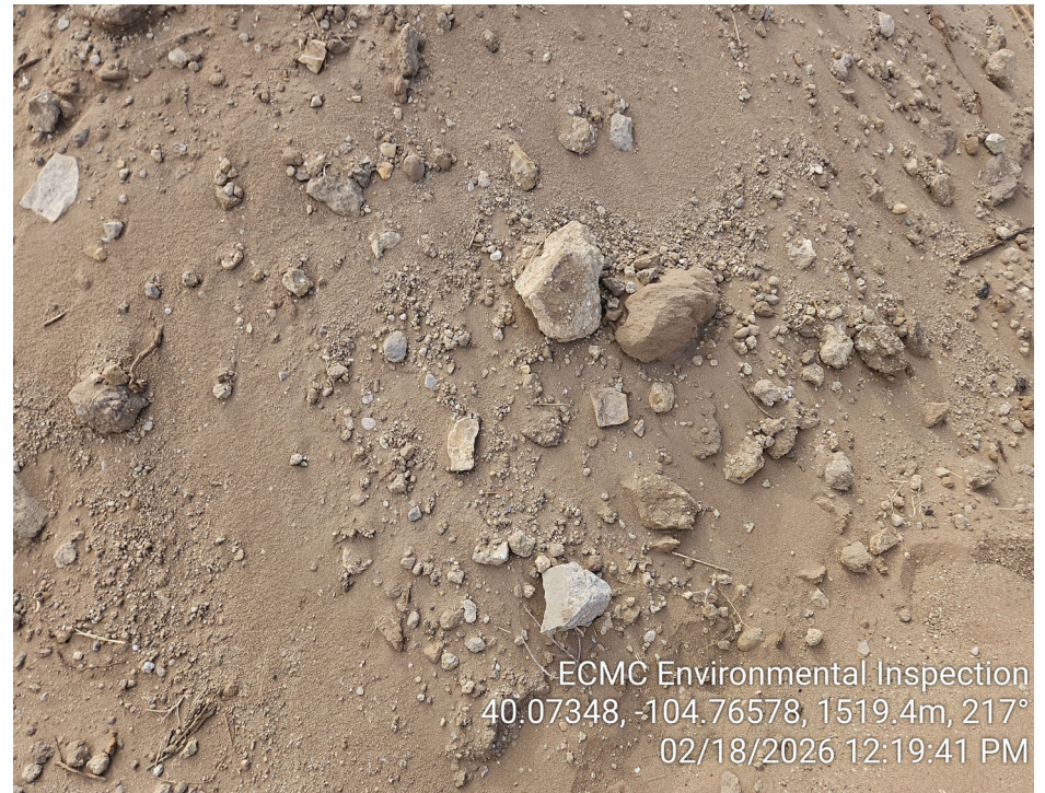
Photo 16 - Soil stockpiles on location for backfill; concrete present in backfill
