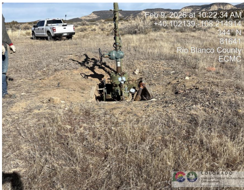
Photo # 1895 Weeds/undesirable plant species on location surrounding production equipment presents a potential fire hazard
