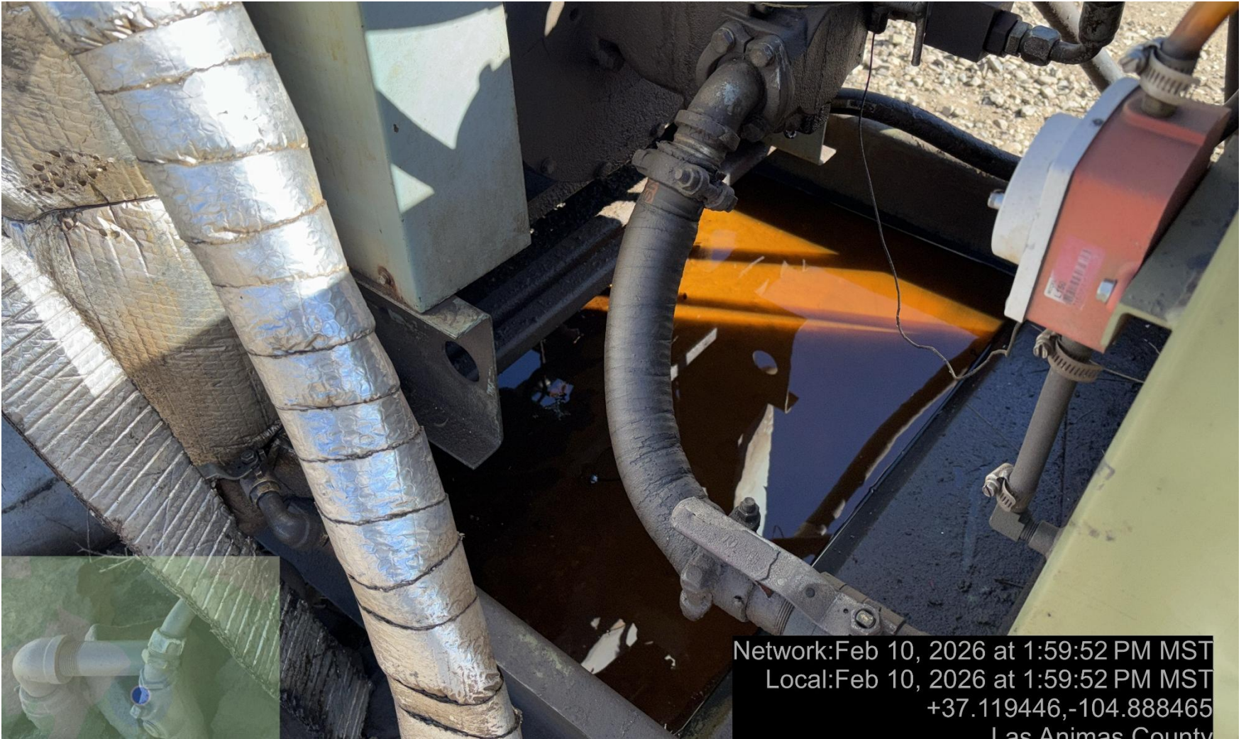
PHOTO 12: OILY WASTE IN PRIME MOVE ENGINE SKID WITHOUT WILDLIFE PROTECTION SCREENS OR COVERS. DRAIN OILY WASTE REPAIR ALL LEAKS AND REMOVE IMPACTED SOIL PER RULE 1002..(2).D & 1002.f.(2)B, Comply with general provisions of the oil and gas act for wildlife protection AND SB-181. immediate action is required, ca date 2/11/2026.
