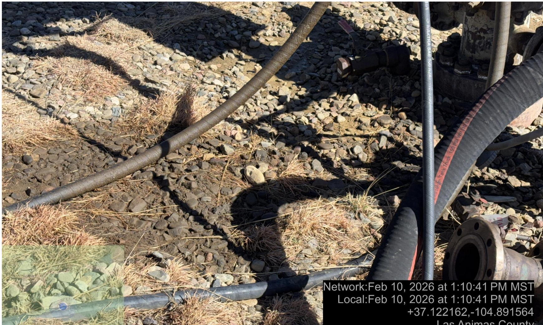
PHOTO 5: area of impacted soil near wellhead appears to be from leaking hydraulic hose. Conduct maintenance on equipment, cleanup stained material and review self inspection processes. COMPLY WITH RULE 1002,(2).D. ca date 2/23/2026.
