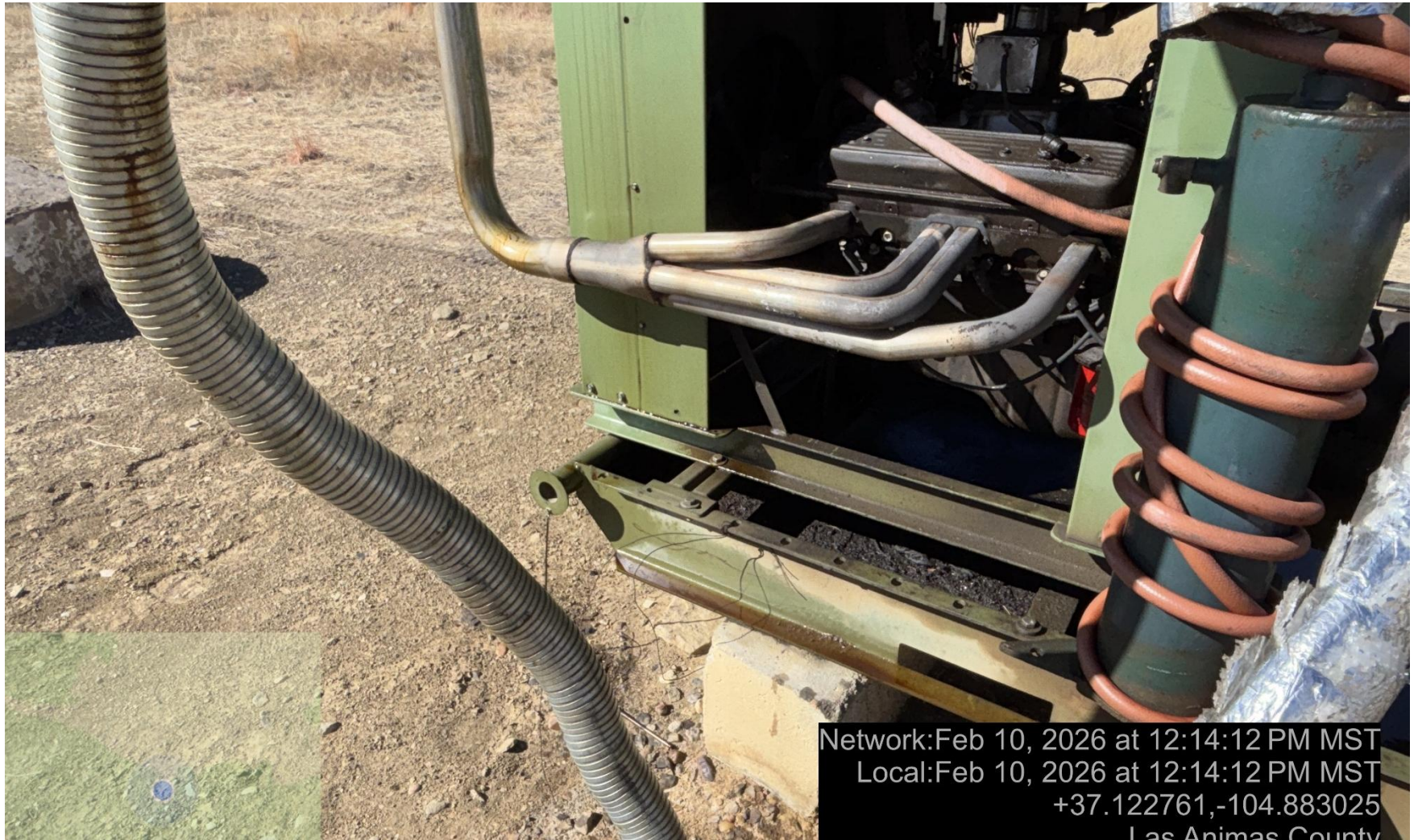
PHOTO 6: area of impacted soil near prime mover skid appears to be used oil leaking out of exhaust. Conduct maintenance on equipment, cleanup stained material and review self inspection processes. COMPLY WITH RULE 1002,(2).D. ca date 2/23/2026.
