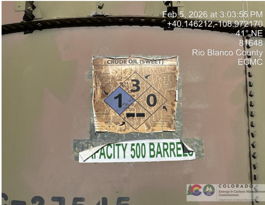
Photo # 1790 Production tank labels not legible & lack required labeling/not in compliance with CECMC rules
