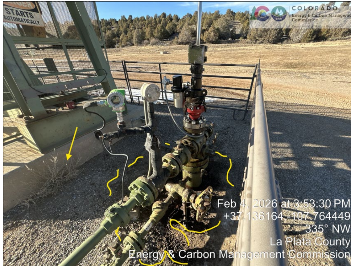
6. Wellhead. Note oil stain on ground (outlined in yellow) and dead vegetative debris (arrow). View looking north. Staining appears to be from excessive rod-oiler lubrication.
