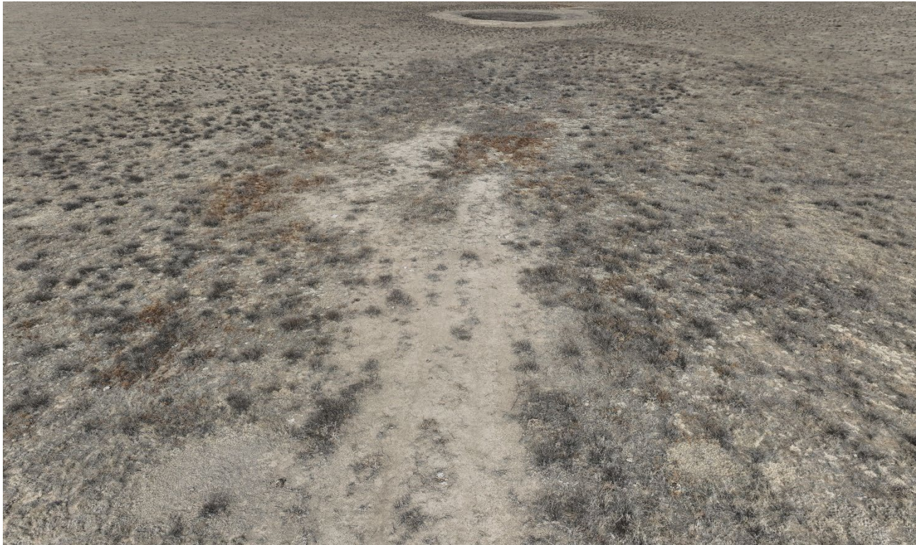
Photo 4. Drone aerial photo facing down toward the abandoned wellsite. There are areas bare of vegetation that need to be reseeded.
