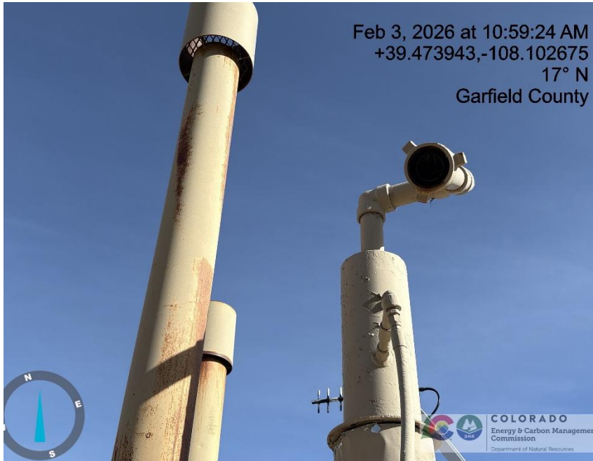
Photo # 8031 Open ended piping on dehy still column /wildlife hazard/available for entry by wildlife
