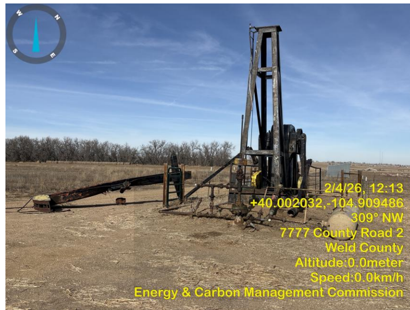
Photo 10 Pump Jack horse head & walking beam have come off the samson post.
