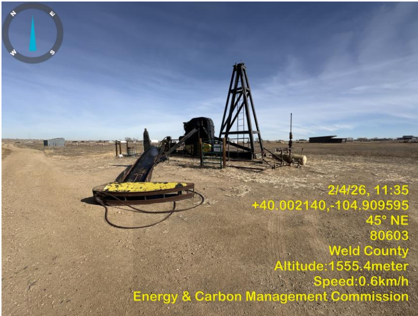
Photo 5 Pump Jack horse head & walking beam have come off the samson post.
