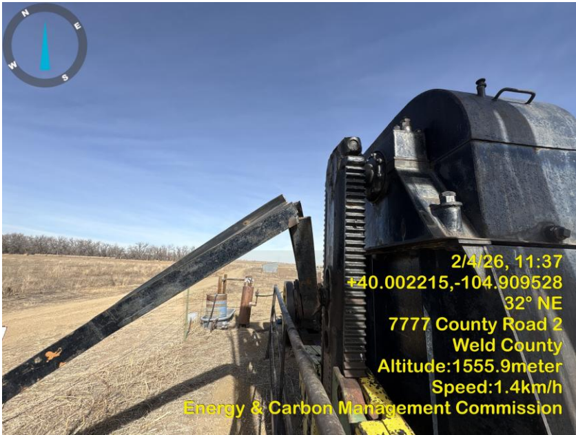
Photo 7 Broken pitman equalizer.
