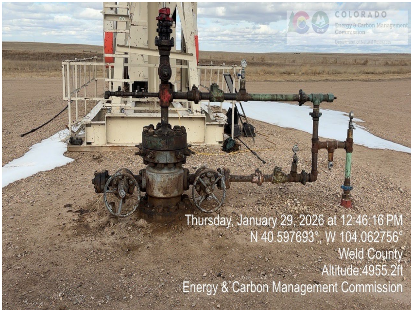
Photo 9 – 2-3H Wellhead – Stained Soil
