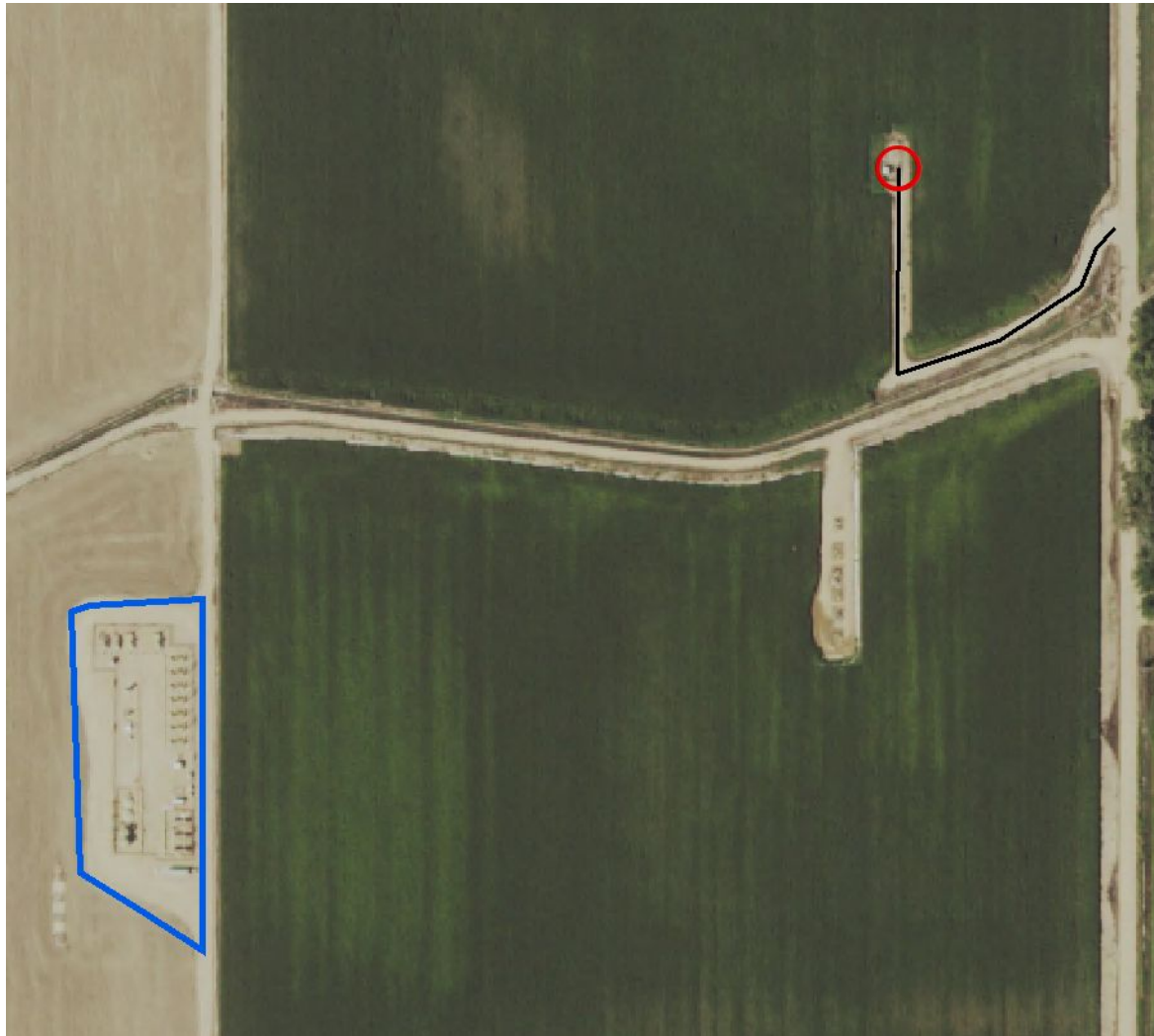
Photo 1. NAIP aerial imagery (2017) illustrating the well location (red circle), associated tank battery location (blue polygon), and access road (black line). The tank battery is associated with location ID #437533.
